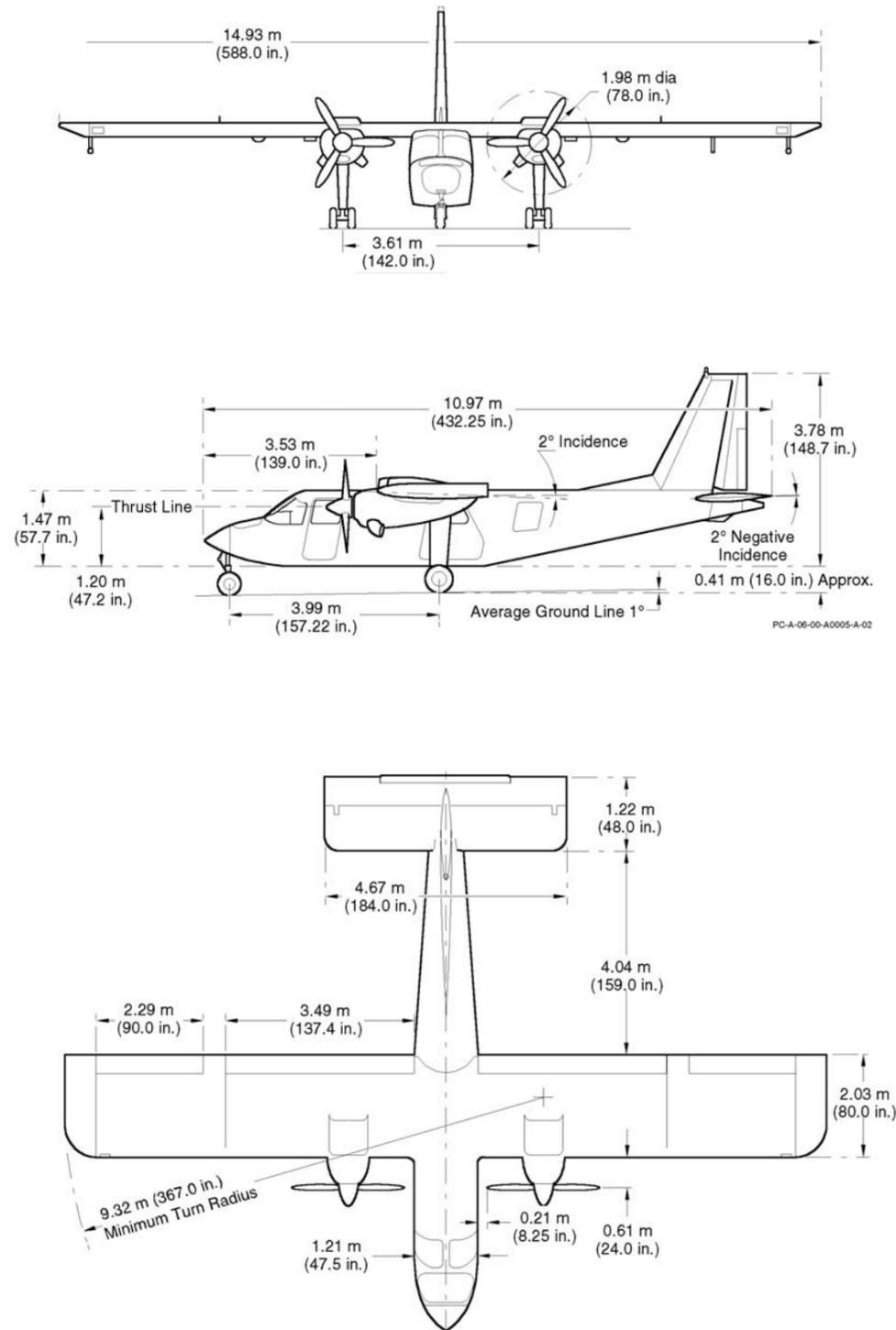
The Britten-Norman Islander is a high wing, twin engine 10 seat monoplane. Three Islander variants are currently available, the 260 and 300hp, BN2B-26 and BN2B-20 Lycoming piston variants and the Rolls Royce turbine engine BN2T. The table below shows the performance comparison between the models.
