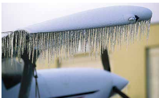
Figure 14.8 Airframe Icing formed on the ground.
