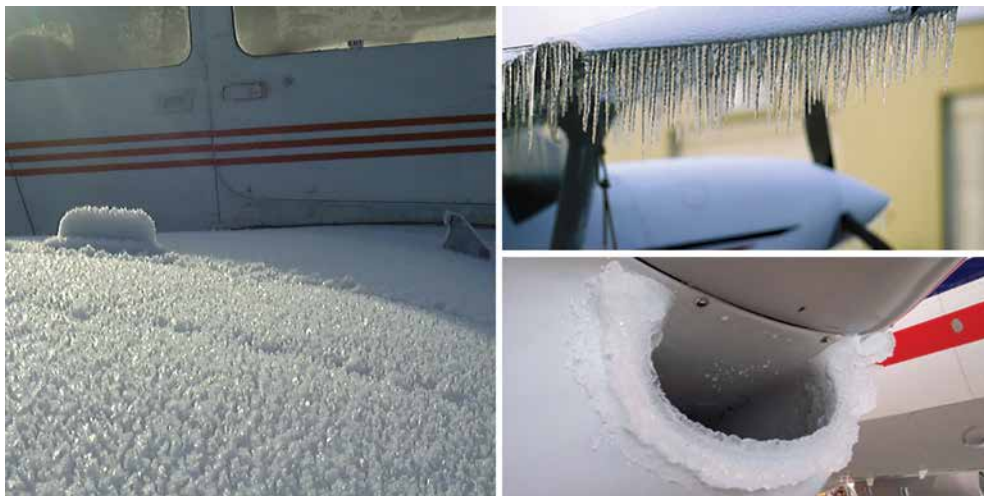
Figure 14.1 Aircraft icing, particularly on the airframe, poses a major hazard to aircraft safety.
