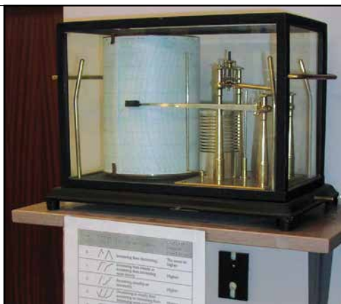
Figure 2.5 A barograph, used to record the variation of air pressure with time, on a cylindrical pressure chart.
