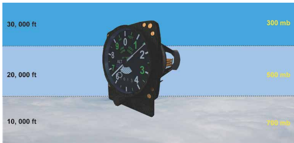
Figure 6.1 Altimetry is based on the fundamental relationship between pressure and altitude. The altimeter is an aneroid barometer calibrated to read height.
