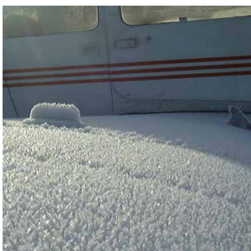
Figure 14.5 Hoar frost on an aircraft's wing.
