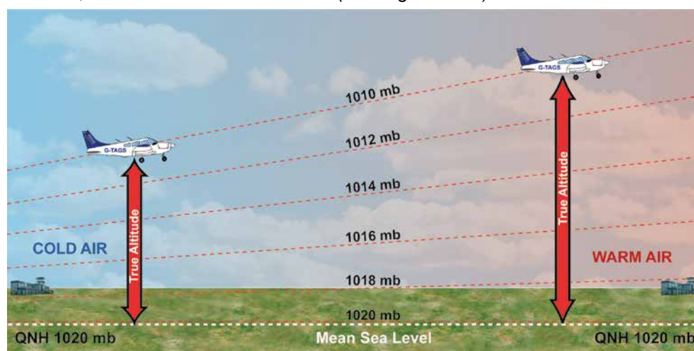
Figure 6.15 When flying from cold air to warm air, the altimeter will under-read.
