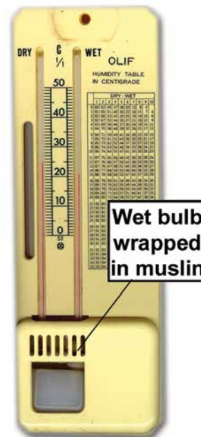
Figure 7.5 A simple hygrometer consists of a wet and dry bulb thermometer.
