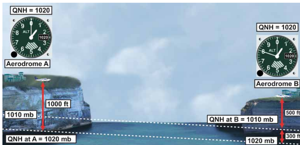
Figure 6.17 Flying from Aerodrome A to Aerodrome B, maintaining an altimeter setting of QNH 1020 millibars (hectopascals).
