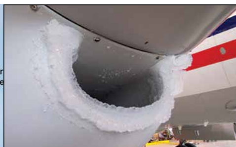
Figure 14.12 Impact ice on engine air intake.
