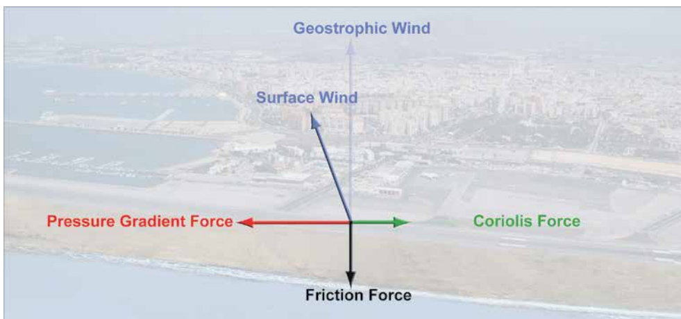
Figure 12.10 Friction will reduce wind speeds. This reduces Coriolis force. The surface wind is deflected towards the Pressure Gradient Force.
