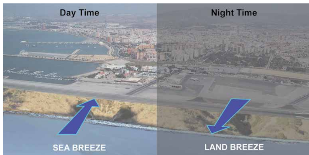
Figure 12.15 The sea breeze and the land breeze will produce a cross wind day and night at this coastal airfield.
