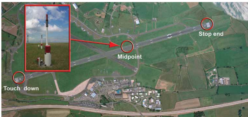
Figure 13.13 RVR (Runway Visual Range) is a reading of visibility along a runway, and is usually measured using a transmissometer.
