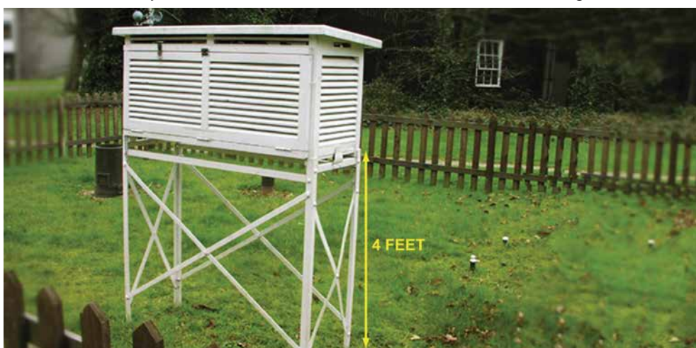
Figure 4.4 Measuring free air temperature: a Stevenson Screen.
