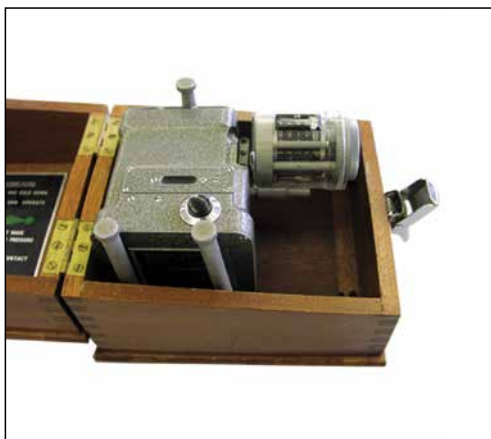
Figure 2.4 A typical aneroid barometer used by Air Traffic Service Units to measure atmospheric pressure at an aerodrome.
