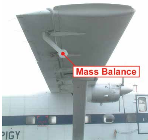
Figure 1.18 A Mass Balance on an aileron.
