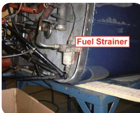
Figure 8.7 Fuel Strainer.
