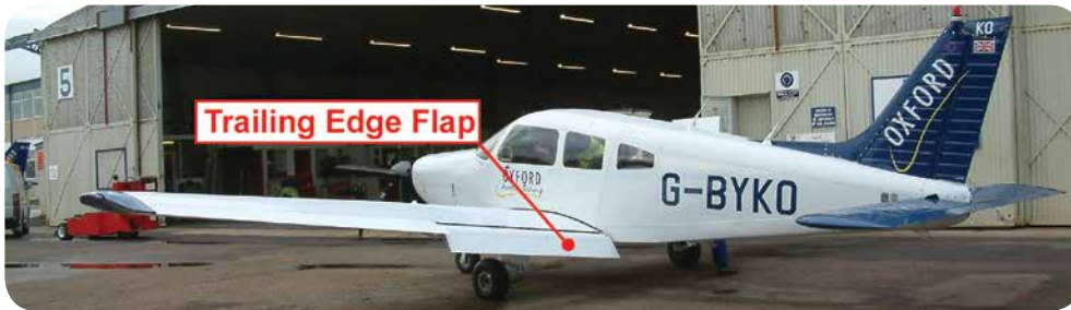
Figure 1.20 Trailing Edge Flaps.
