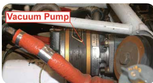
Figure 12.1 An Engine Driven Vacuum Pump.
