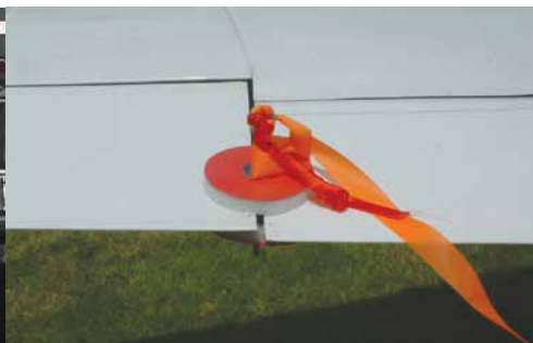
Figure 1.26 Externally Fitted Control Lock.
