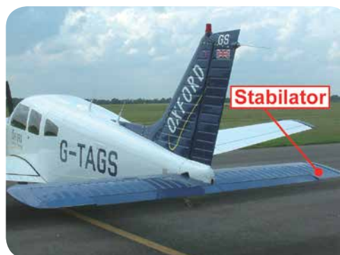
Figure 1.23 The Stabilator.
