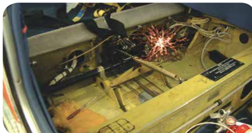
Figure 11.17 Electrical Faults May Cause Fires.
