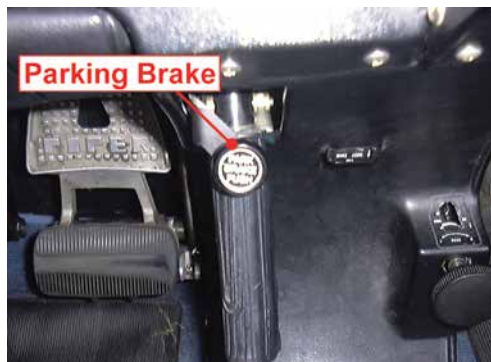
Figure 10.3 Parking Brake.
