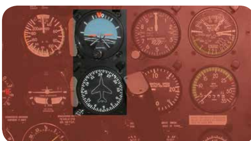
Figure 12.2 The Direction Indicator and the Attitude Indicator.
