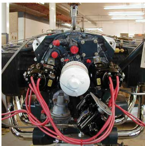
Figure 3.13 The Accessory Housing.
