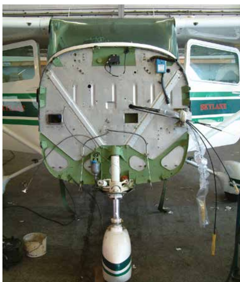
Figure 1.5. An Engine Bulkhead.
