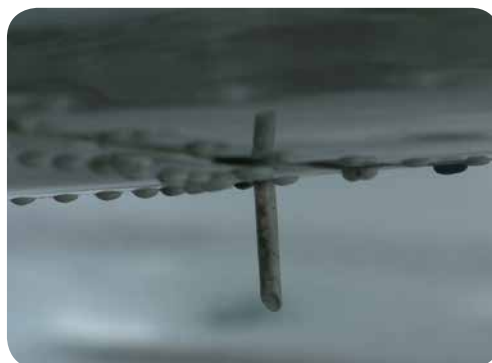
Figure 8.6 Fuel Tank Vent.
