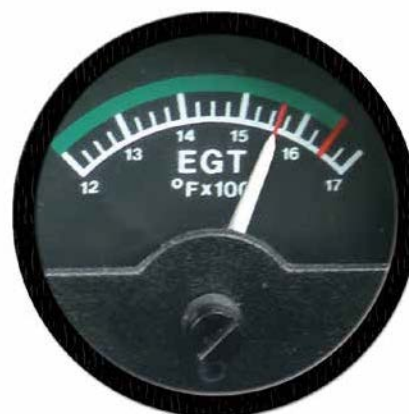
Figure 13.4 An EGT Gauge - graduated in degrees Fahrenheit.
