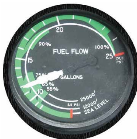
Figure 13.14 A Fuel Flowmeter.
