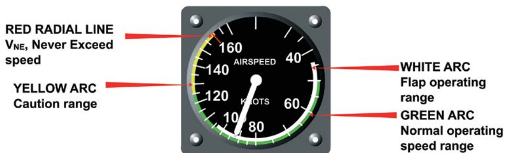
Figure 14.11 Colour Coding on the Airspeed Indicator.
