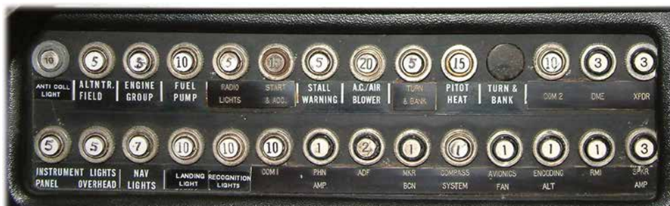
Figure 11.18. An Aircraft Circuit-Breaker Panel.
