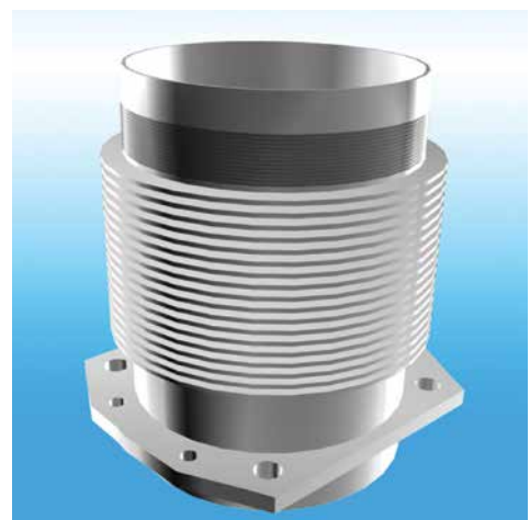
Figure 4.4 The cylinder is finned to increase the cooling area.
