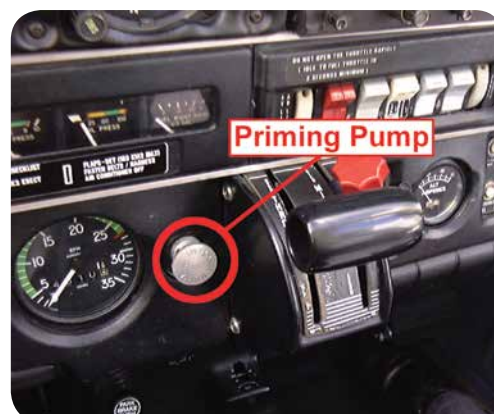
Figure 10.6 The Priming Pump.
