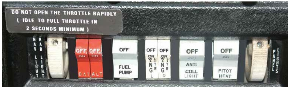
Figure 11.22. Power Switches in a PA 28 Aircraft.
