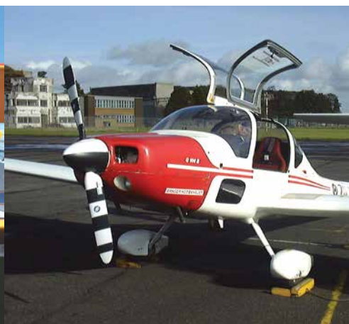
Figure 9.17 A Two-Pitch Propeller.
