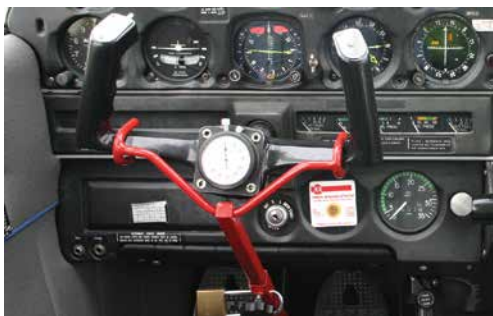
Figure 1.25 Internally Fitted Control Lock.
