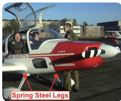
Figure 2.3 Spring Steel Legs.
