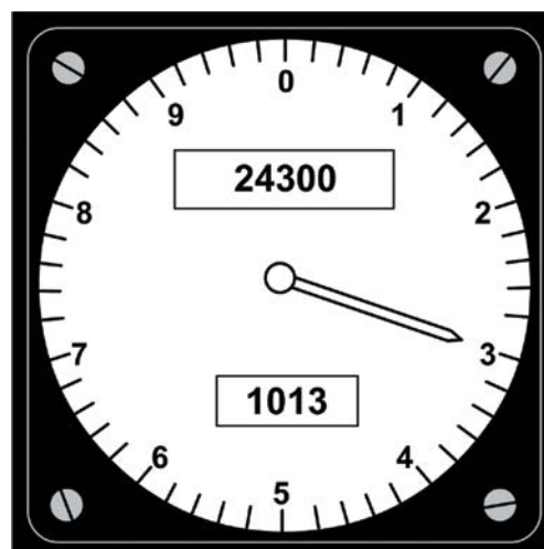
Figure 14.17 Counter Pointer Altimeter.
