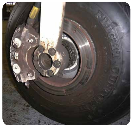
Figure 2.18. An Aircraft Disc Brake Assembly.
