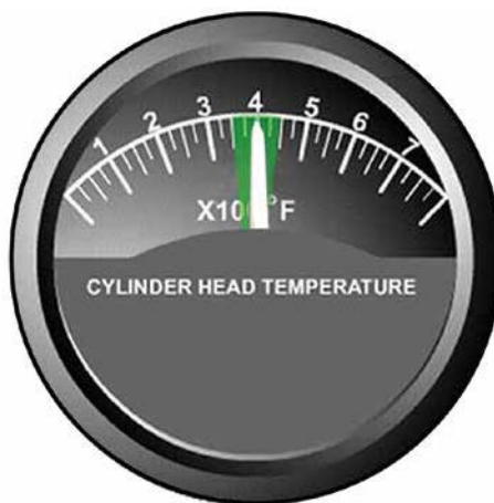
Figure 13.5 A Cylinder Head Temperature Gauge.
