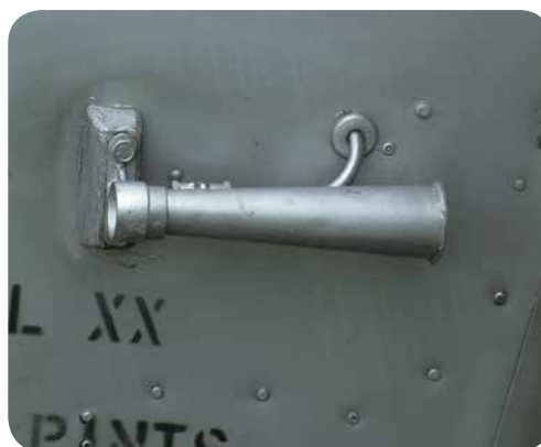
Figure 12.4 A Venturi Tube and suction tube on an Auster Mk6.
