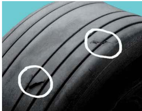
Figure 2.13. Cuts in the Tread of a Tyre.
