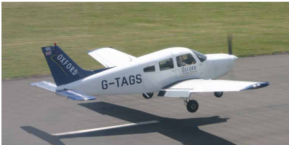
Figure 1.5 Maximum Landing Mass (MLM) is the maximum permissible total mass of the aircraft on landing, under normal circumstances.
