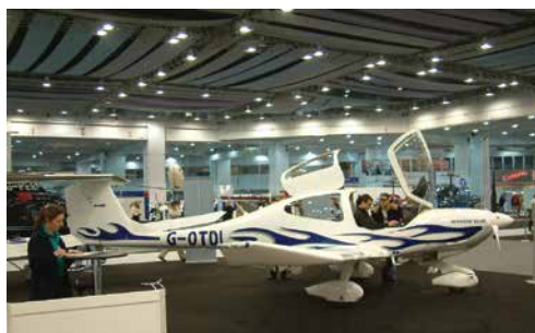
Figure 11.8 The Airframe of this Diamond Star is made of non-conductive materials.
