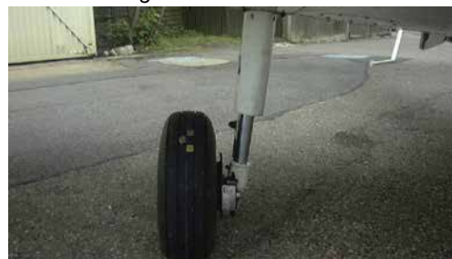
Figure 2.5 An Oleo-Pneumatic Strut.
