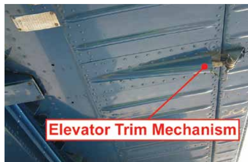
Figure 1.19 Elevator Trim Mechanism.
