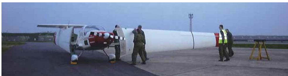
Figure 16.9 Replacing Wings which are Designed for Disassembly.
