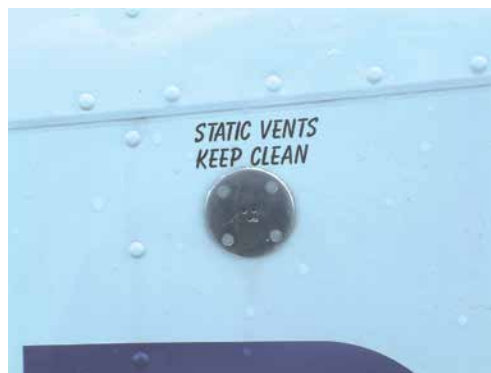
Figure 14.6 A Static Vent.
