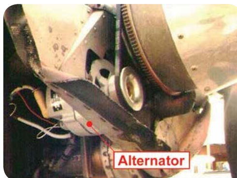
Figure 11.9 An Alternator.
