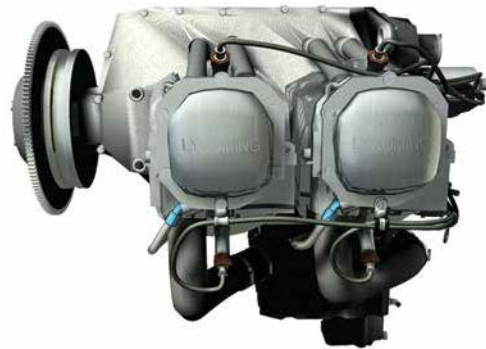
Figure 5.3 A Wet-Sump Engine.
