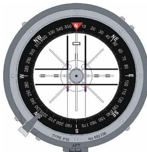
Figure 15.19 The Grid Ring Compass.
