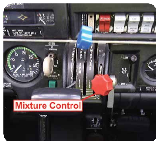
Figure 10.10 The Mixture Control.
