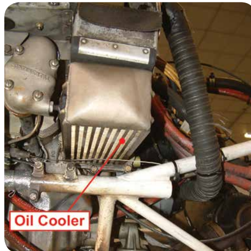
Figure 5.1 An Oil Cooler.
