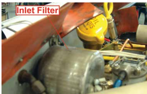
Figure 12.7 An Inlet Filter.
