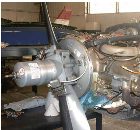
Figure 9.18 Constant-Speed Propeller.
