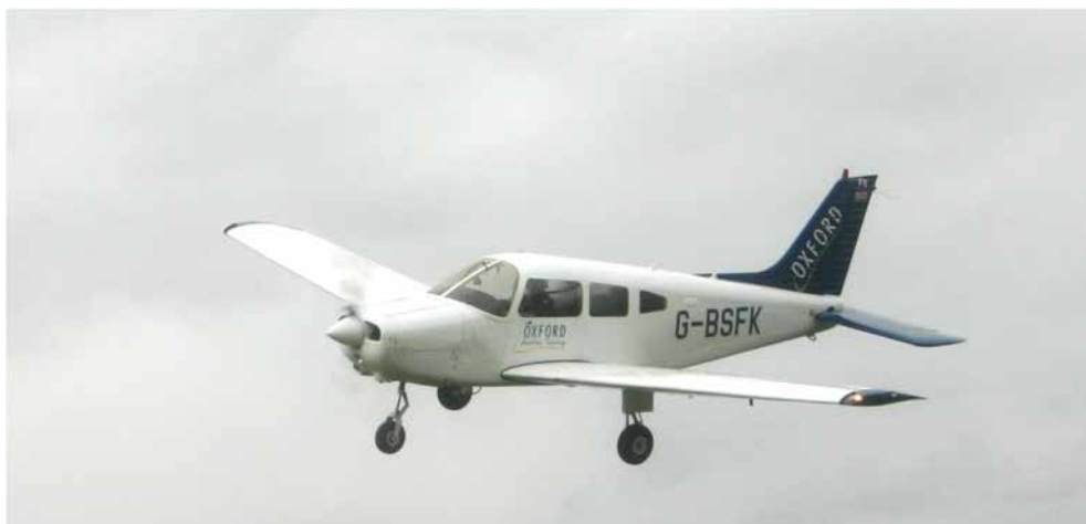
Figure 2.18 The Warrior can operate either in the Normal or Utility Categories, depending on its operating mass.
