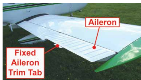
Figure 1.16 An Aileron.
