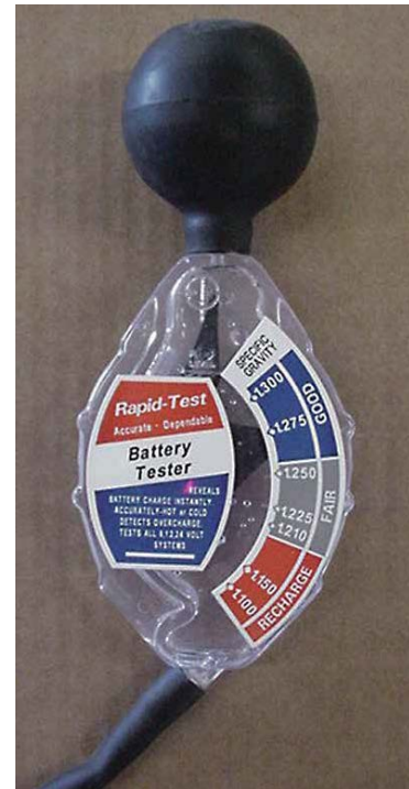
Figure 11.12 An Hydrometer.
