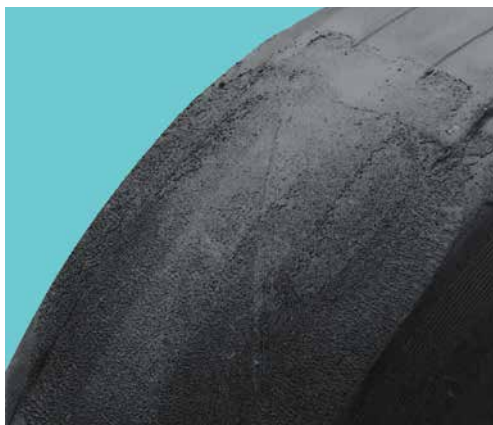
Figure 2.17. A Tyre Damaged by Aquaplaning.
