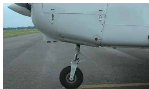
Figure 2.7 Nose Gear.
