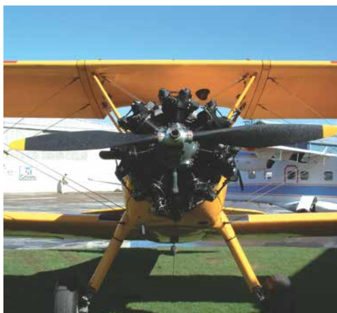
Figure 9.16 Adjustable-Pitch Propeller.
