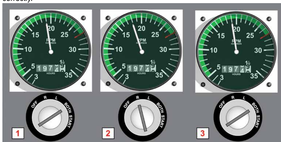
Figure 10.8 Checking the right-hand magneto; 1 = both on, 2 = right on only, 3 = back to both.
