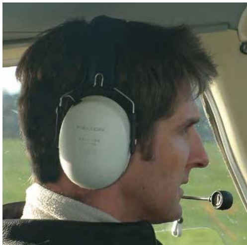
Figure 2.1 Here, the microphone is too far from the pilot's lips.
