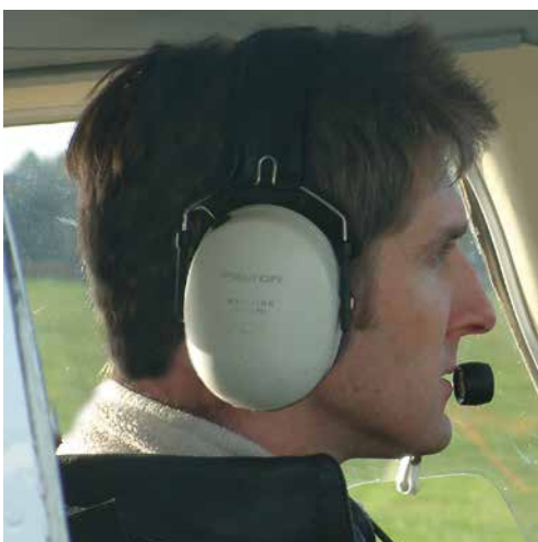
Figure 2.2 Here, the microphone is too close to the pilot's lips.
