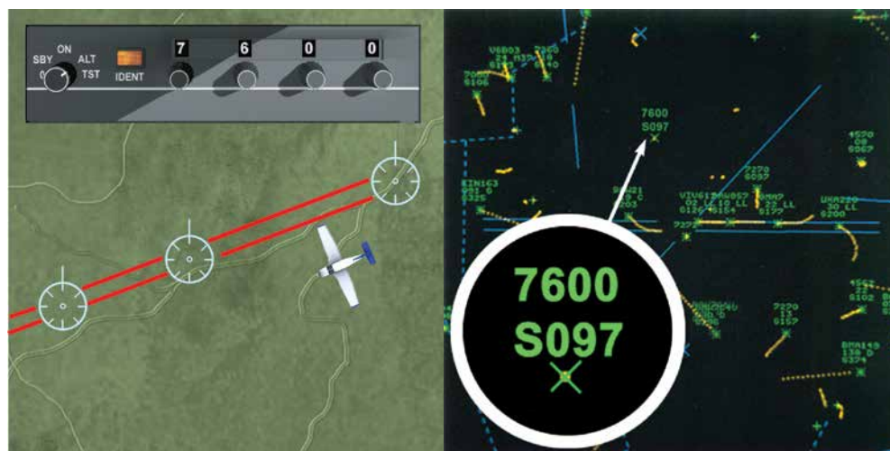
Figure 8.2 If you experience communications failure, and your aircraft is equipped with a transponder, squawk 7600.
