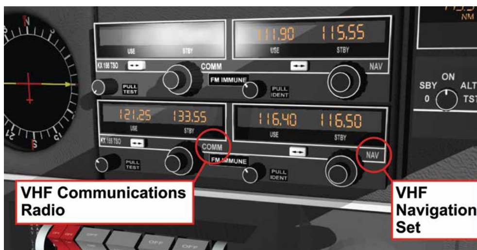
Figure 1.1 VHF Communications and VHF Navigation Sets fitted to a light aircraft.
