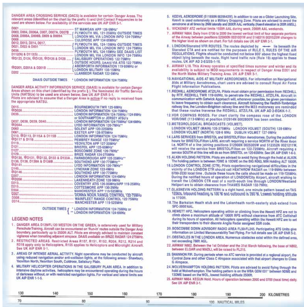
Figure 13.6 Frequencies to contact for UK Danger Area Crossing Service and the Danger Area Activity Information Service may be found on the UK 1:500 000 Aeronautical Charts.
