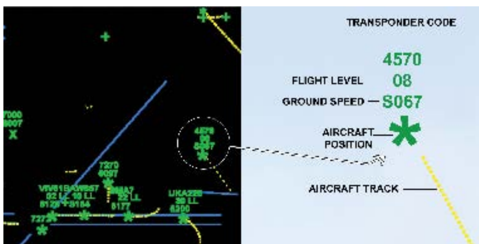
Figure 7.8 A typical ATC Radar display, with SSR enhanced traces.
