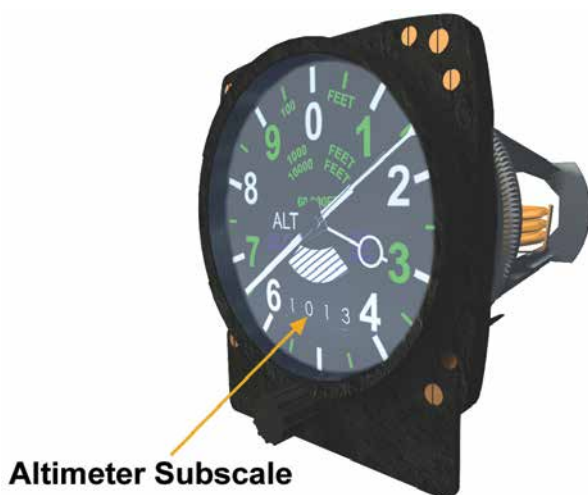
Figure 19.1 The altimeter subscale set to the Standard Pressure Setting of 1013 mb.
