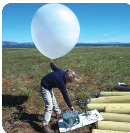
Figure 18.11 Radiosonde balloon launch.
