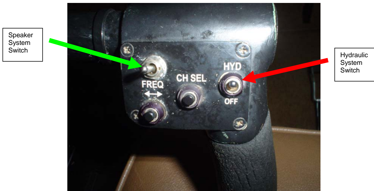
Figure 4: The green arrow indicates to the speaker system switch. The red arrow indicates to the hydraulic switch on the cyclic control stick. Note that the 2 switches look exactly the same.
