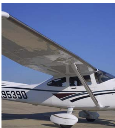
Porous Panels on Wing and Lift Strut
