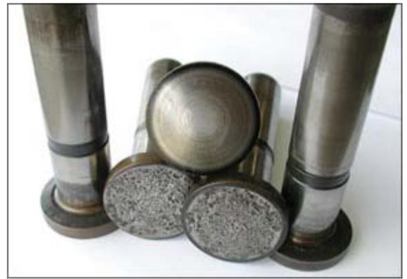
The cam destruction shown here begins with micro-pitting caused by corrosion, as shown on the lifters in bottom photo. Engine oil's role is to prevent the corrosion in the first place and fresh oil does that better than dirty oil.
