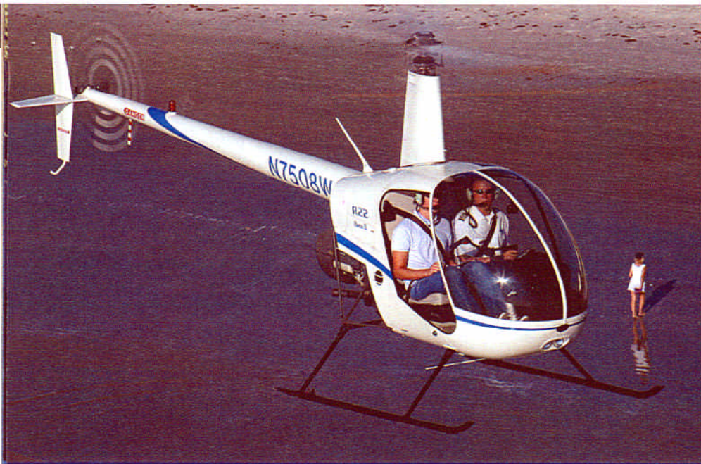
■ (left) The R22 shines with a 102 kts VNe, and a cruise speed of 96 kts at 70% power.
