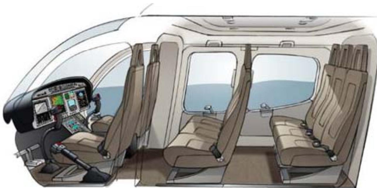
Standard Six Place Passenger Seating – Airline Arrangement
