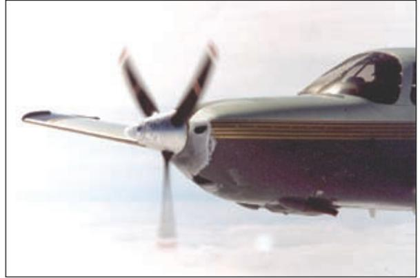
400 equipped with the electrothermal E-Vade system: "During the three years that I have flown with E-Vade I have had about six icing encounters. E-Vade failed completely in three. It worked partially in one, with most panels working fine, but with at least one panel failing to heat and allowing ice to accumulate.
